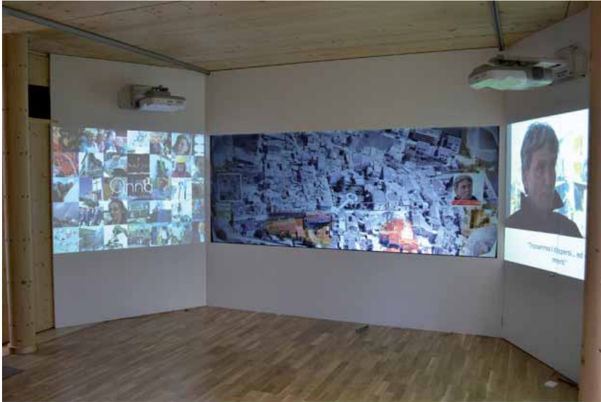
Fig.1- the installation is composed of a central interactive rear-projected screen and two lateral screens used for displaying non-interactive multimedia contents
