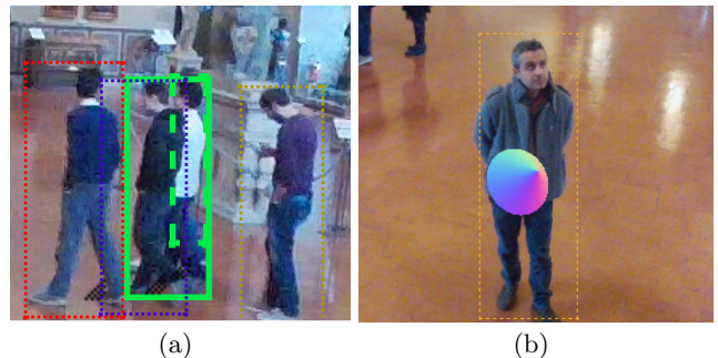
Figure 3: (a) The solid green rectangle represent the bounding box selected for the annotation while the green dashed rectangle represent the visible (not occluded) area annotated by the user; (b) The cone visualizes the annotation of the gaze provided by the user.
