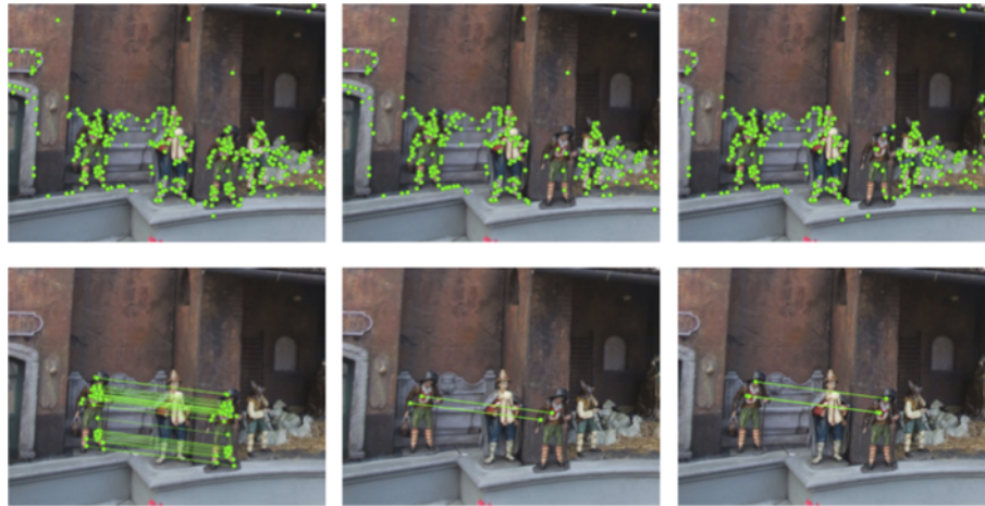
Figure 9 Example of copy-move removal-injection attack (2). Extracted keypoints (top) and SIFT matches (bottom) for image Nativity : copy-move attack without keypoint removal (left), with keypoint removal (middle), and with keypoint removal-injection (right).
