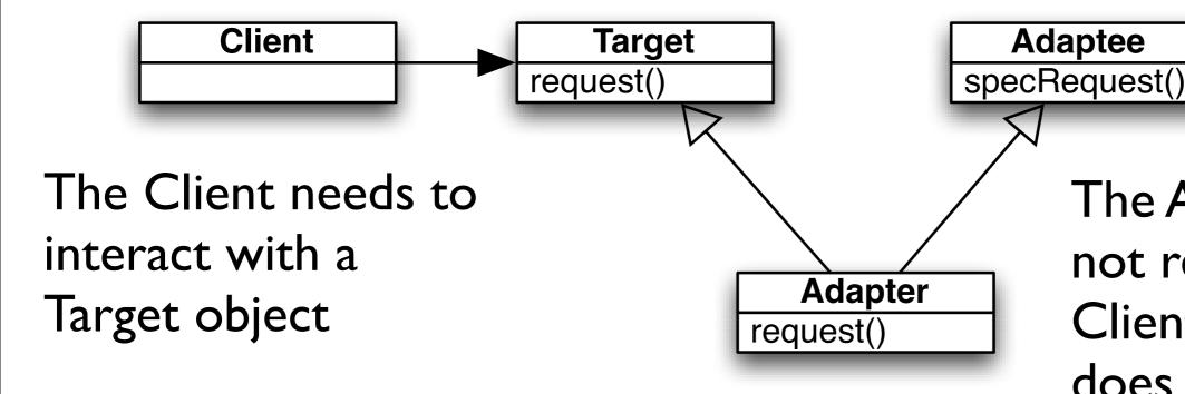
The Adaptee could not respond to Client because it does not have the required method
