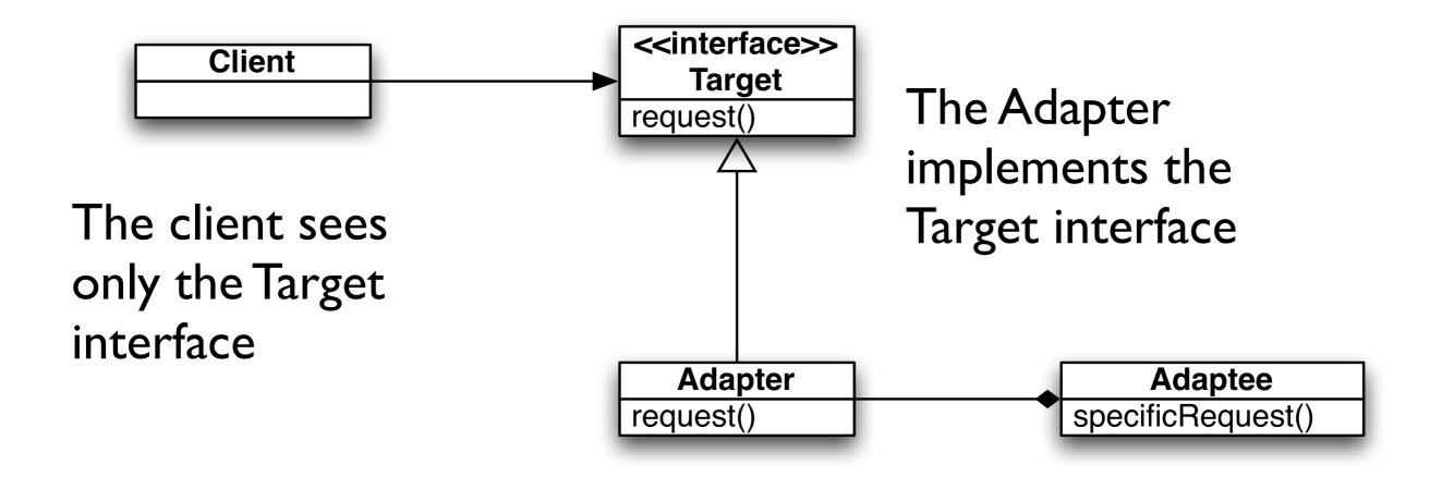
The Adapter is composed with the Adaptee
