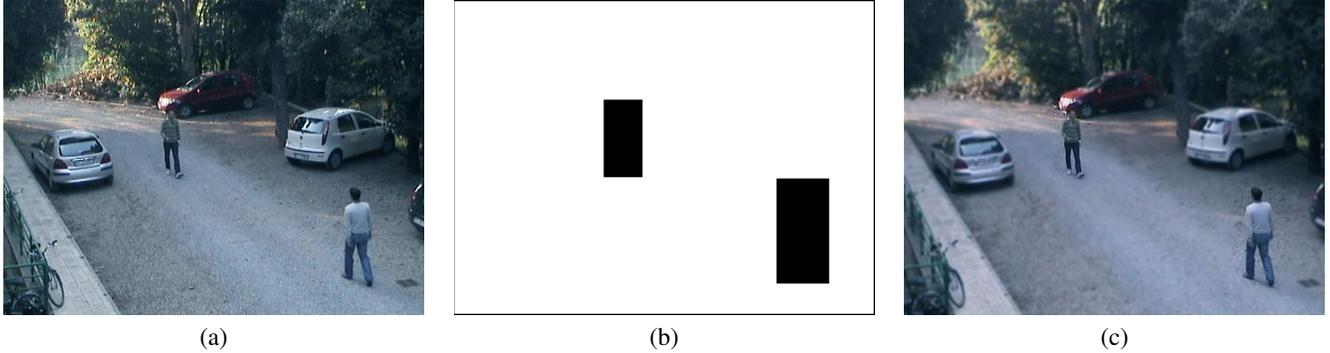
**Fig. 4.** Adaptive compression driven by pedestrian detector. A frame with two people (a), the masks built with the pedestrian detector (b) and the final adaptively encoded frame (c). All the scene but the two pedestrian is smoothed.
