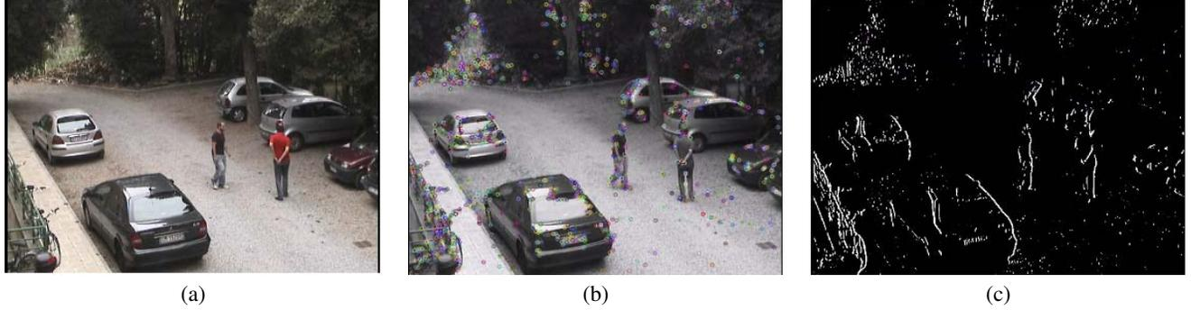
**Fig. 2.** Examples of the features used for adaptive image encoding. (a) The original video frame. (b) Corners points detected using the FAST detector. (c) Edges detected using the Sobel gradient operator. Note how both the corner and edge features tend to be concentrated on and around the semantically relevant objects in the scene: people, cars, license plates, etc.
