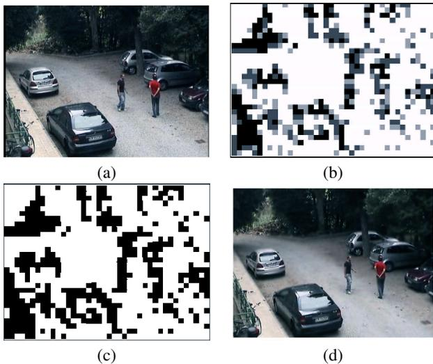
**Fig. 3.** An example of feature-preserving adaptive compression. (a) Original video frame. (b) The multi-level mask computed from FAST and Sobel responses. (c) A single level mask from FAST and Sobel features. (d) The frame compressed using the single-level mask. Note how persons and license plates are encoded with high enough quality to preserve recognizability, while background details are smoothed away.
