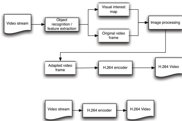
**Fig. 1.** Our approach to adaptive video coding. (top) The schema for semantic video adaptation. (bottom) standard video coding.
