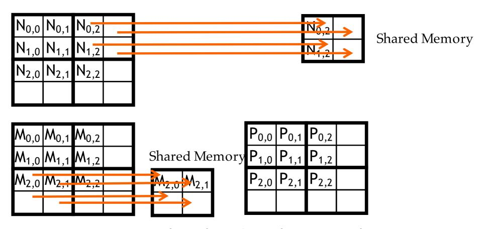
Threads (1,0) and (1,1) need special treatment in loading M tile
