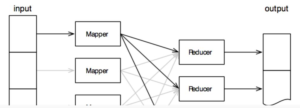
"Map" step: Each worker node applies the "map()" function to the local data, and writes the output to a temporary storage. A master node orchestrates that for redundant copies of input data, only one is processed.
