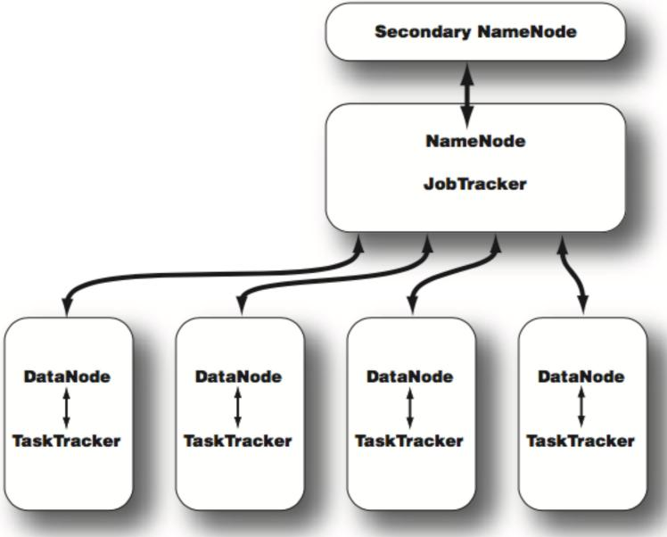
Topology of a typical Hadoop cluster. It's a master/slave architecture in which the NameNode and JobTracker are masters and the DataNodes and TaskTrackers are slaves.
