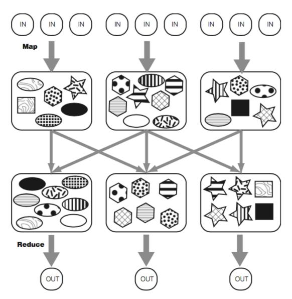
The MapReduce data flow - partitioning and shuffling. Each icon is a key/value pair. The shapes represents keys, whereas the inner patterns represent values. After shuffling, all icons of the same shape (key) are in the same reducer. Different keys can go to the same reducer, as seen in the rightmost reducer. The partitioner decides which key goes where. Note that the leftmost reducer has more load due to more data under the "ellipse" key.
