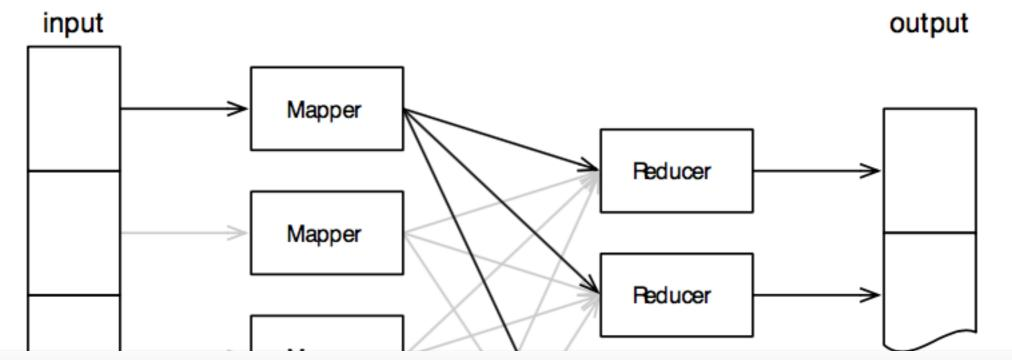
"Map" step: Each worker node applies the "map()" function to the local data, and writes the output to a temporary storage. A master node orchestrates that for redundant copies of input data, only one is processed.
