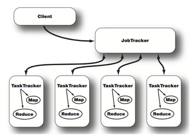
JobTracker and TaskTracker interaction. After a client calls the JobTracker to begin a data processing job, the JobTracker partitions the work and assigns different map and reduce tasks to each TaskTracker in the cluster.
