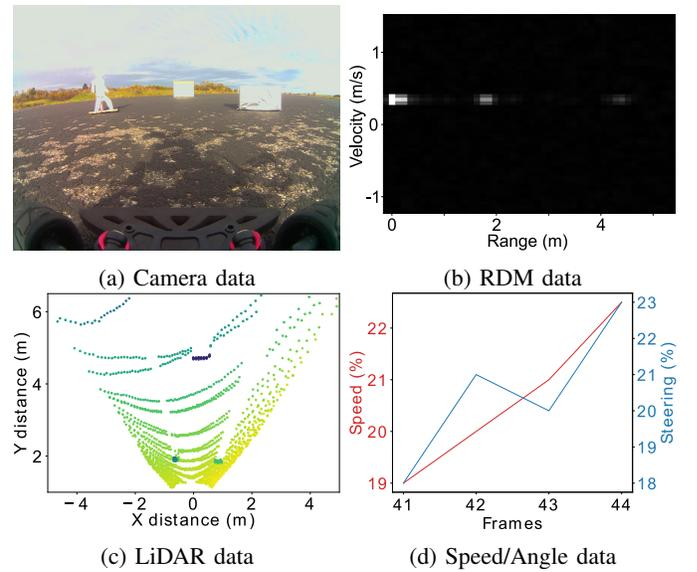
Fig. 3: Frame sample of camera, radar, LiDAR and Speed/Steering data.
