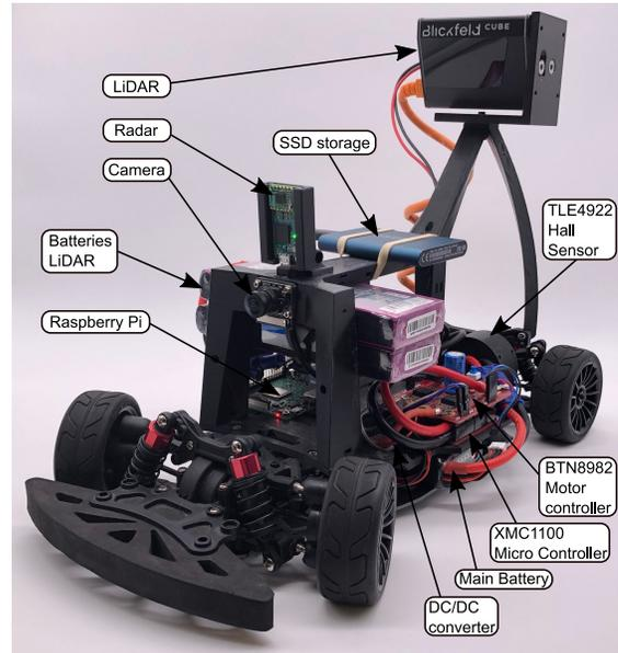
Fig. 1: Developed RC car system
