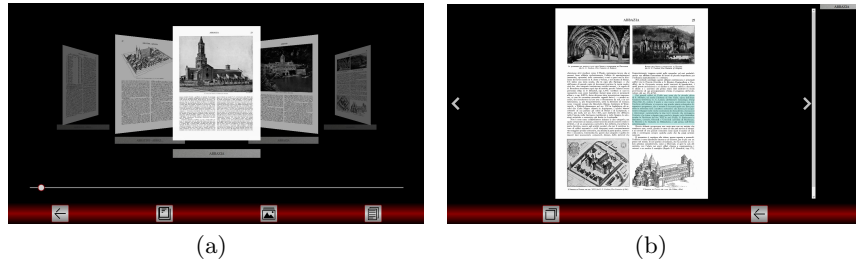
Fig. 5. Displaying a page in the visualization interface. The page content is highlighted in blue when the cursor hovers on it.
