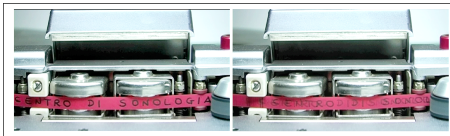
Fig. 3. Test for video shooting. On the left, a correct setting of the camera: each frame is clear and the text is readable. On the right, a wrong setting of the camera. The aim is to detect physical defects of the tape (due to aging or joints) that may correspond to a specific noise in the audio signal. Audio is directly recorded from a secondary line-out of the STUDER A-810.
