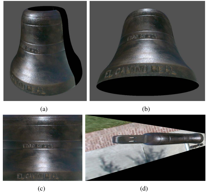
Fig. 6. Applications. (a),(b): two synthetic views of the reconstructed bell of Fig. 1. (c): metric flattened texture of the bell surface (the imaged cross-section looks straight). (d): metric rectification of the floor inferred from the SOR.
