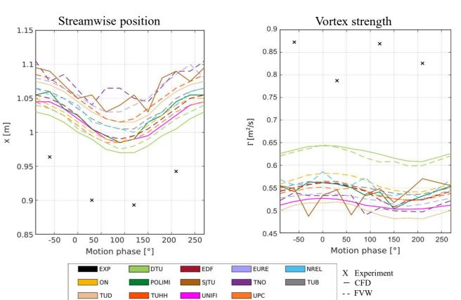
A sinusoidal motion of the platform induces oscillations in the tip vortex position and strength. The strength oscillations are in a 90° delay compared to the streamwise position.
