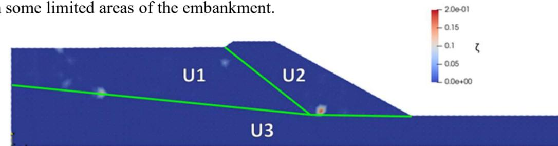
**Fig 2.** Liquefaction potential evaluation through effective stress ratio  $\zeta$ .
