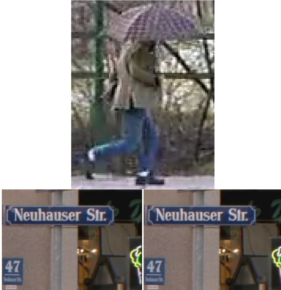
Fig. 1: Examples of video compression artifacts: top ) blocking artifacts on the bottom part of the green pole, color interpolation due to chroma sub-sampling on left and right of the umbrella; mid ) and bottom ) ringing around the white on blue text in the street name sign; little vertical flickering (1-2 lines) of numbers and letters (in particular N and 7) between two following frames.
