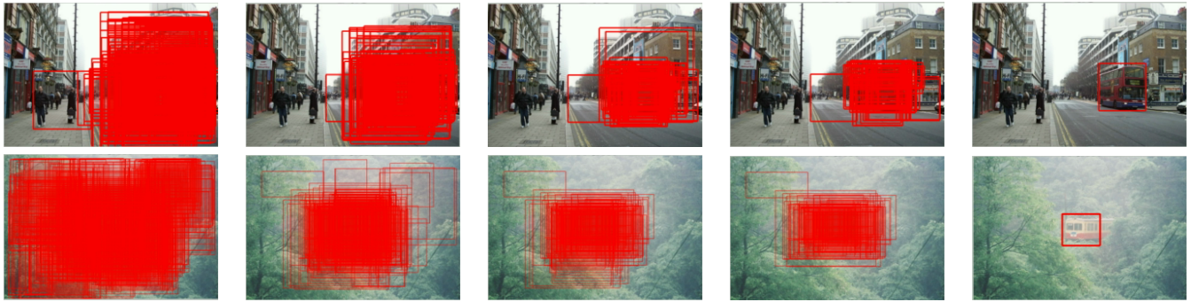
Fig. 3. Windows retained during tree traversal using rejection thresholds. The amount of windows decreases significantly from the first tree node (leftmost) to the last (rightmost).
