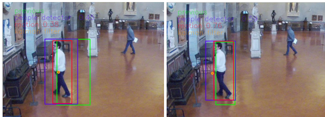
Figure 5: Example of annotation prediction for two consecutive frames. Bounding box in the previous frame (green solid line), bounding box generated using motion detection (red solid line), bounding box obtained through pedestrian detection (blue solid line), the position predicted with the Kalman filter (orange circle).
