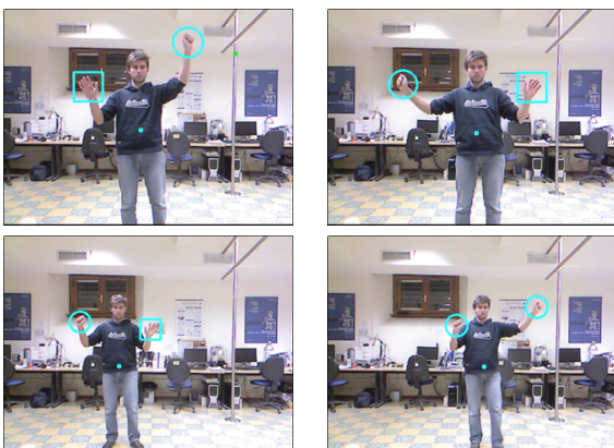
Figure 6. Hand status detection: square (open hand), circle (closed hand).
