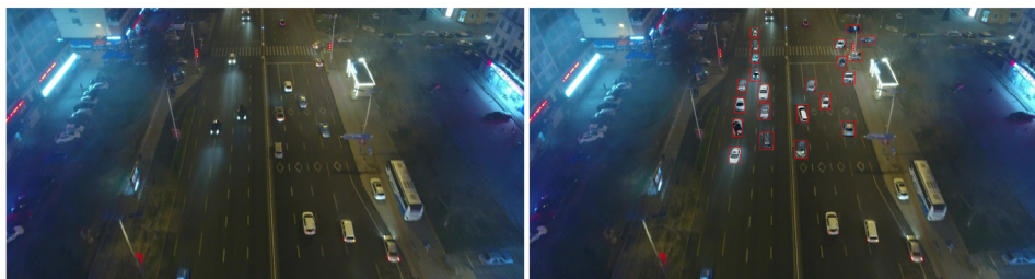
Fig. 1. We describe a pipeline for small object data augmentation able to populate an original frame (left) with new generated small objects (right), highlighted in red. (For interpretation of the references to colour in this figure legend, the reader is referred to the web version of this article.)
