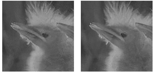
Fig. 3: Left: reconstruction without sub-patch strategy. Right: our sub-patch strategy reduces mosquito noise and ringing artifacts.
