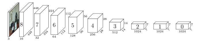
Figure 2: Our network architecture, with tensor size and layer numbering.
