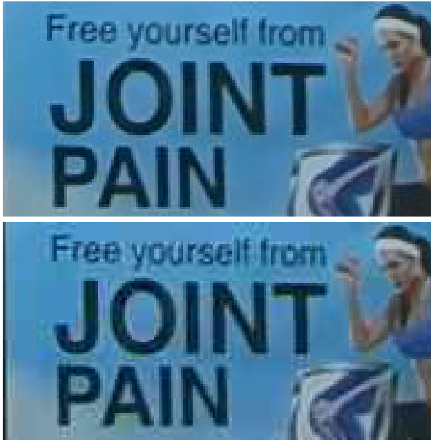
Figure 2: Examples of compression artifacts in text images. Top row: high quality image; bottom row: low quality compressed image. Ringing artifacts are visible on all letters, color deviation and blurring are more visible on the borders of the vertical strokes of P, I, N and T. Artifacts affect both versions of the image. Best viewed in color and zoomed in.
