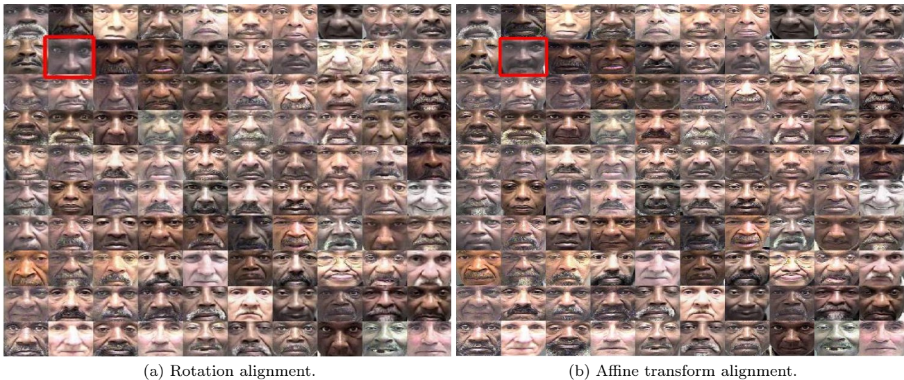
Fig. 3: Alignment results with rotation compensation and with affine alignment. In the face marked in red the mouth is missing in the rotated image whilst using the affine compensation all important facial features are visible.
