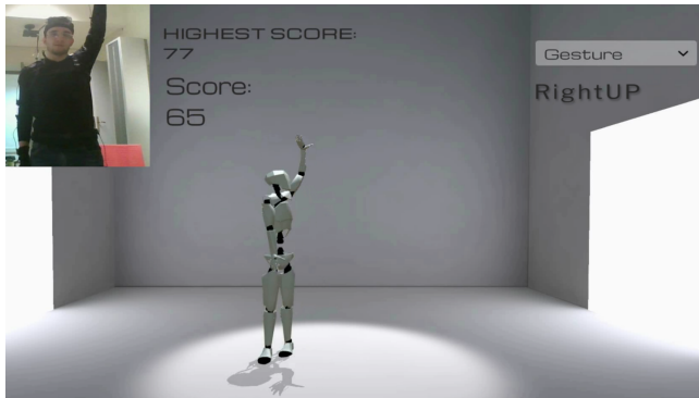
Figure 2: In recognition mode gestures and poses are automatically recognized in real time. Gesture recognition can be exploited in Unity or by other applications through the standalone tool.
