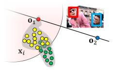
Figure 5. Matching with multiple identities. The identity  $o_1$  matches with two identities (yellow and green). The ambiguity is resolved by assigning  $o_1$  with the Id having the largest number of matched descriptors (i.e. the yellow identity).
