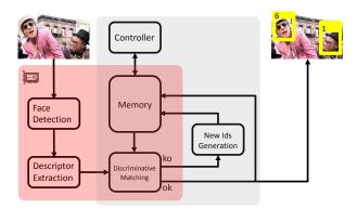
Figure 2. Block diagram presenting the major work flow and functional components in the proposed method. The gray shaded region highlights the components discussed in this paper. The memory module and the matching strategy run on the GPU.
