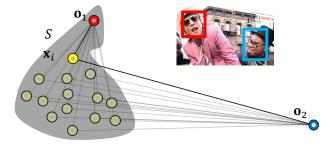
Figure 3. Reverse Nearest Neighbor for a repeated temporal visual structure (S) with the distance ratio criterion. All elements  $\mathbf{x}_i$  match with  $\mathbf{o}_1$ , for clarity only one of them is highlighted to show the distances (thick black lines).
